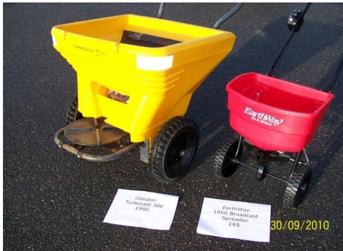
WSCC recommends a spread rate of **approximately 20 grams of salt / grit per metres square** when hand salting. Although salt/grit can be spread effectively with shovels, care is required to ensure over salting does not occur. Push-along devices as shown above can be used to cover larger areas with an even spread. Large areas can thus be treated quicker with less wastage.
